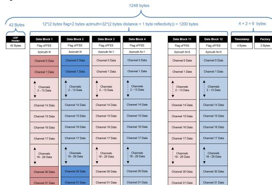
Figure 9-3 VLP-32 Dual Return Mode Data Structure
