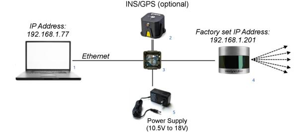
Figure 2-1 Example 3D Sensing System
