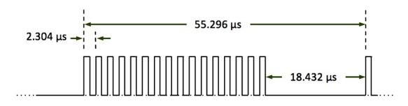
VLP-32C lasers are fired in pairs at widely separated angles to minimize IR crosstalk. The sequence of firings is specified in *Table 9-5 below*. The first pair to fire is lasers 0 and 1. The second are 2 and 3. And so on.
