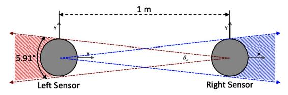
The angle subtended by the shadow of a sensor in range but at some distance from another sensor is given by the following formula:
