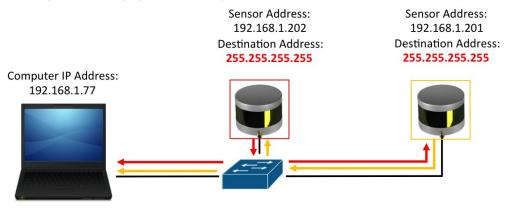
J.2.3.2 Multiple Sensors Transmitting to a Specific Address
