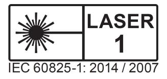
**Note:** The VLP-32C sensor is a CLASS 1 LASER PRODUCT. The product fulfills the requirements of IEC 60825-1:2014 (Safety of Laser Products).
