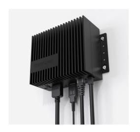
The Stereolabs ZED Box is an industrial AI gateway offering powerful edge computing capabilities for autonomous robotics and spatial analytics. Specifically designed to use with the ZED-2 and ZED-2i cameras, it is powered by an NVIDIA® Jetson™ embedded GPU, enabling deployment of state-of-the art AI and 3D vision solutions.
