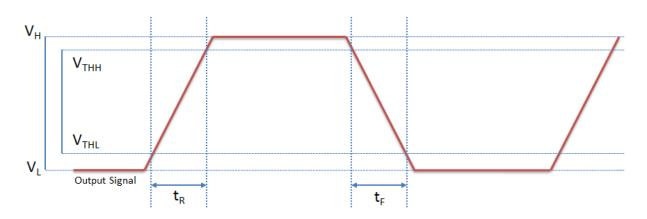
Figure 6.5: Opto-isolated output timing characteristics
