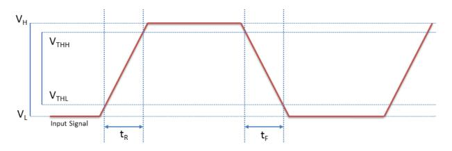
Figure 6.7: Non-isolated input timing characteristics
