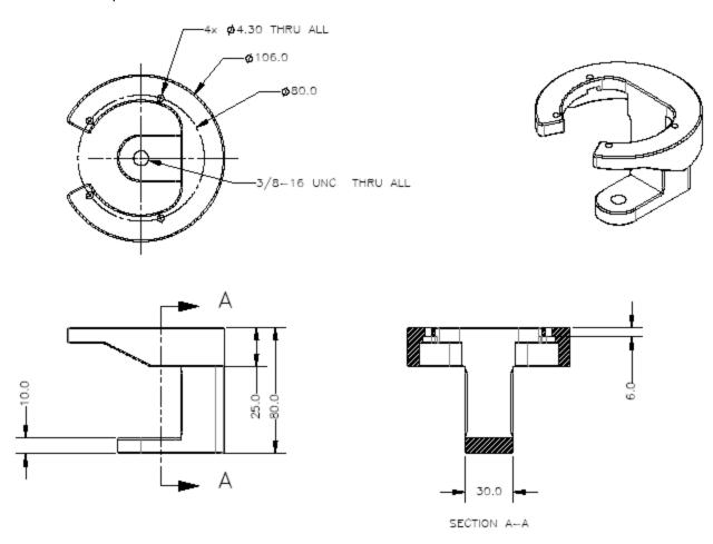
Figure 4.3: Tripod Adapter (in mm)
