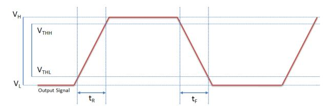
Figure 6.8: Non-isolated output timing characteristics
