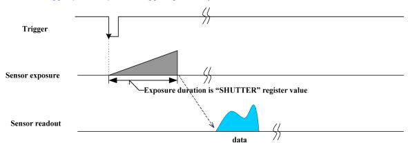
Figure 7.1: Trigger Mode 0 ("Standard External Trigger Mode")
