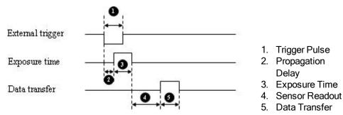
Figure 7.5: External trigger timing characteristics
