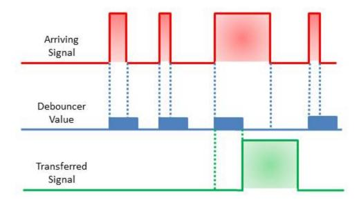
Figure 6.1: Debouncer Filtering Invalid Signals
