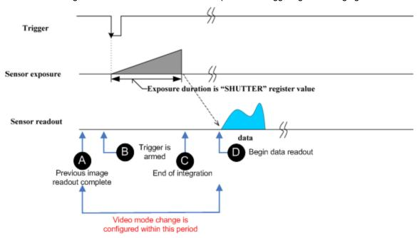
Figure 7.6: Relationship Between External Triggering and Video Mode Change Request
