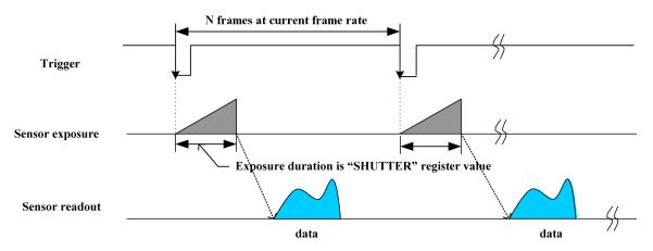
Figure 7.2: Trigger Mode 3 ("Skip Frames Mode")
