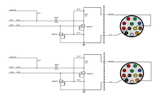
Figure 6.6: Non-Isolated input and output GPIO circuit
