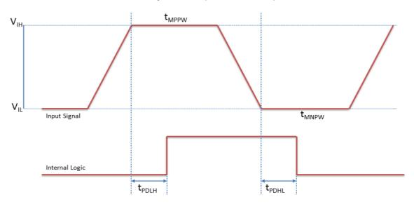
Figure 6.4: Opto-isolated input timing characteristics
