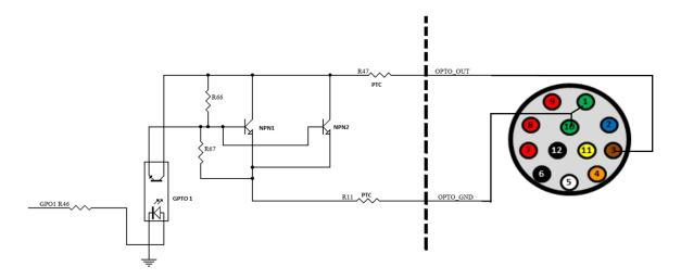
Figure 6.3: Opto-isolated output circuit
