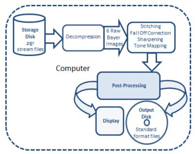
Figure 1.2: Ladybug5 post processing workflow
