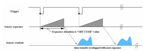
Figure 7.3: Trigger Mode 14 ("Overlapped Exposure/Readout Mode")
